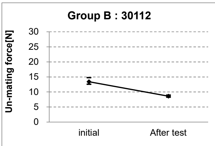
Graph3. Part No.30112 unmating force
