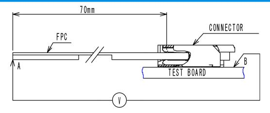
Contact Resistance  $= R_{AB} - Resistance$  of a 70mm length of FPC cable.
