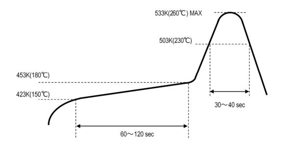
Fig. 1 Reflow Temperature Profile
