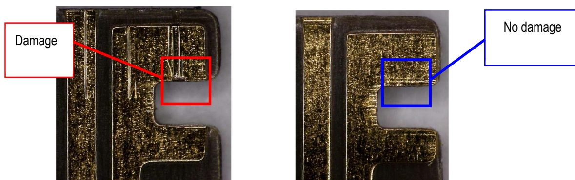
Fig.24 In case withdrawing FPC with (a) actuator close condition or (b) actuator release condition
