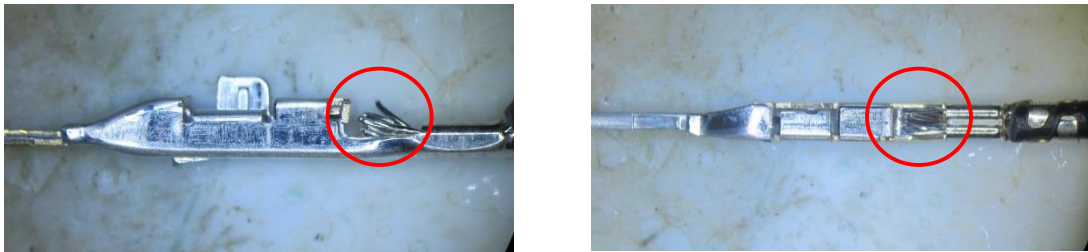
Fig 19 Excessive conductors out
