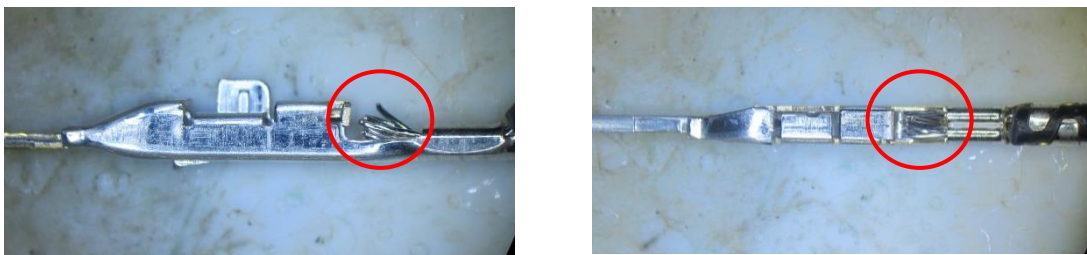
Fig 19 Excessive conductors out
