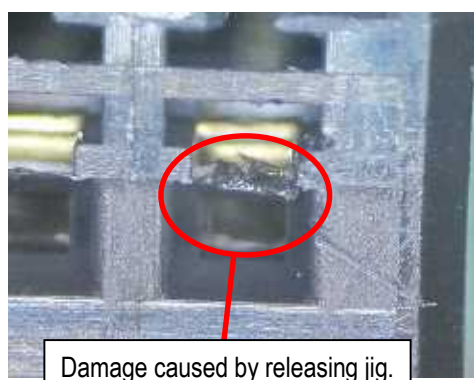
Fig42 Damage caused by releasing jig
