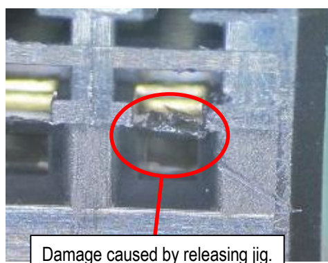
Fig41 Damage caused by releasing jig
