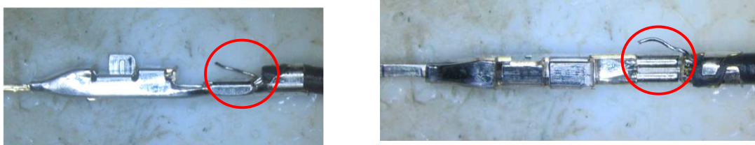
Fig 20. Incomplete conductors crimping
