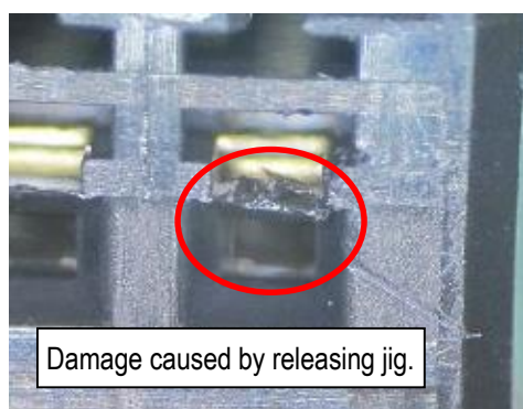
Fig35. Damage caused by releasing jig
