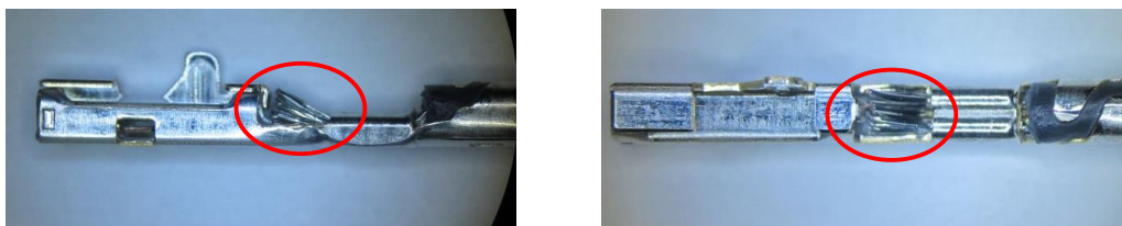
Fig 19 Excessive conductors out
