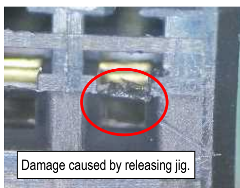
Fig36.Damage caused by releasing jig
