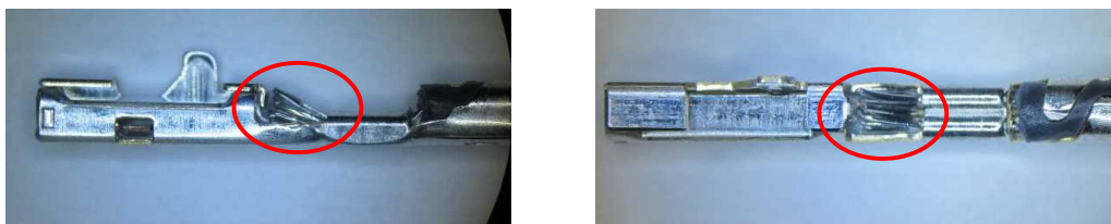
Fig 19 Excessive conductors out
