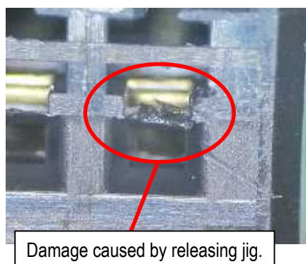
Fig.41 Damage caused by releasing jig
