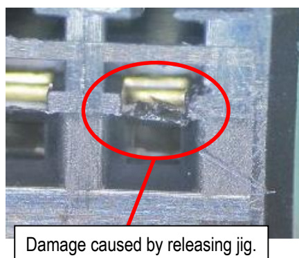
Fig.40 Damage caused by releasing jig
