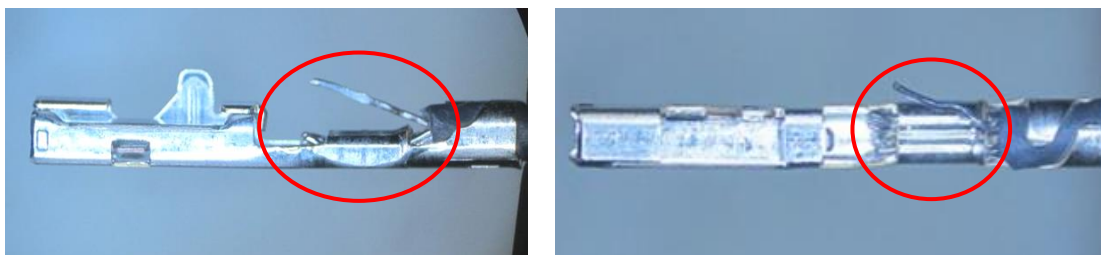
Fig.22 Incomplete conductors crimping
