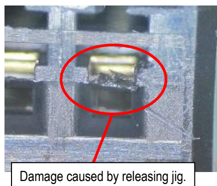
Fig.41 Damage caused by releasing jig
