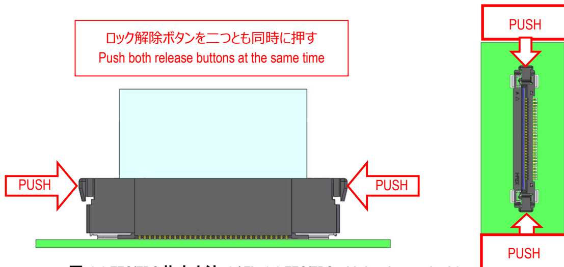
図. 3-2 FFC/FPC 抜去方法 2 / Fig.3-2 FFC/FPC withdrawing method 2
