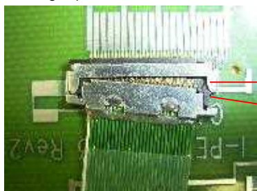
10°こじり状態 / 10°Chape condition
