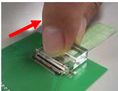
平行抜去 OK 状態 / parallel pull out OK condition
