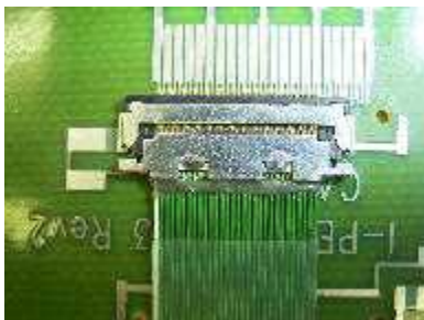
仮差し状態 / Temporarily condition
