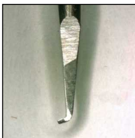
【Reference】 The Tip of Pull Jig (For withdrawing the one side of connector)
