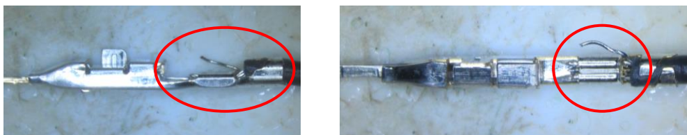
図/ Fig 20.端子はみ出し状態/ Incomplete conductors crimping
