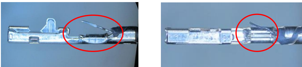
図/ Fig 20.芯線はみ出し状態/ Incomplete conductors crimping
