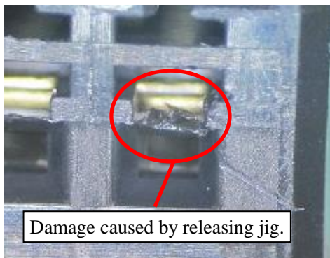
Fig34. Damage caused by releasing jig
