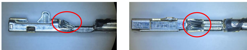
Fig 17 Excessive conductors out
