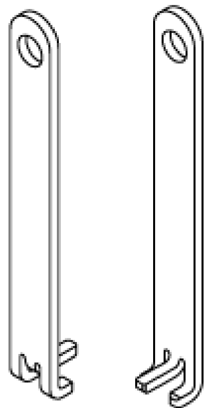
FRONT SIDE BACK SIDE MHF I MATING AND UNMATING TOOL PART NO. 90224-001
