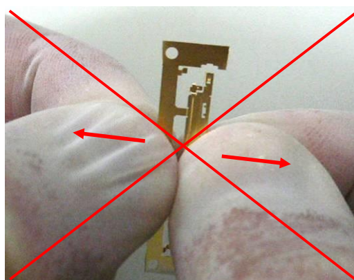
Photo.10 Cut by Force (Bad Example)
