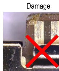
Photo 8. Incorrect FPC condition
