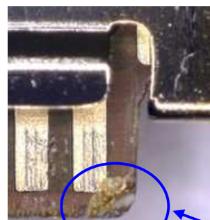
Fig 6. FPC insertion - Bad example 2
