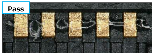
Photo. 1 After applying flux
