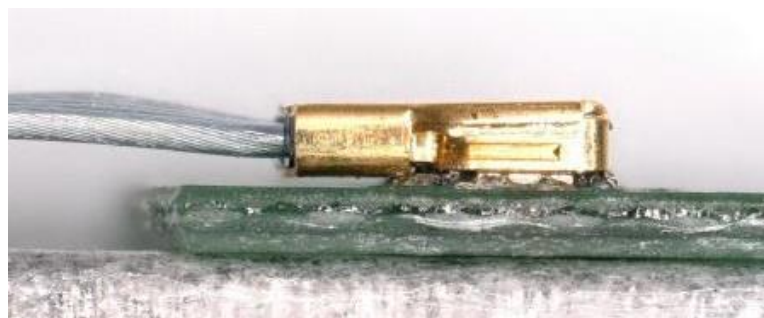
Photo. 38 Crimping height OK
