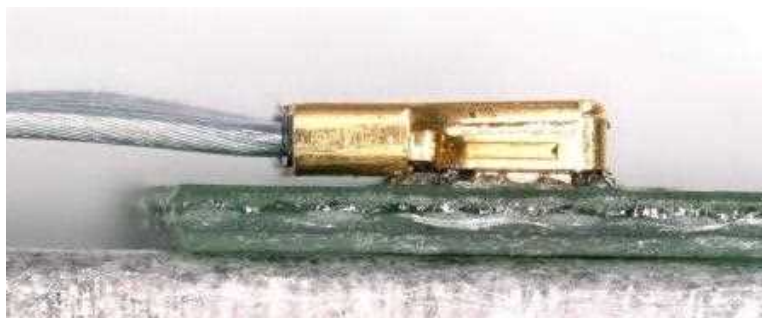
Photo. 28 Crimping height OK
