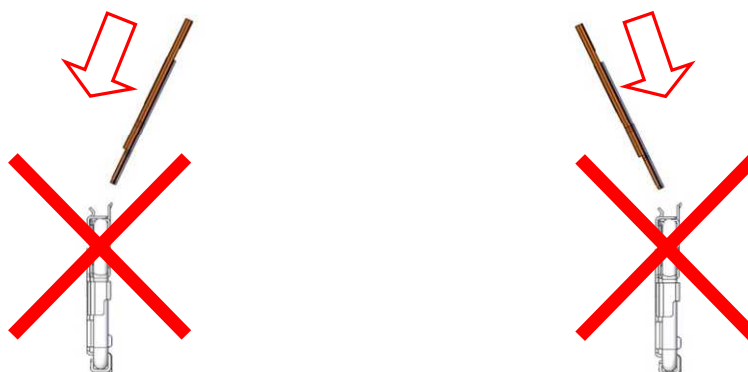
Fig.6 Slanted FPC insertion
