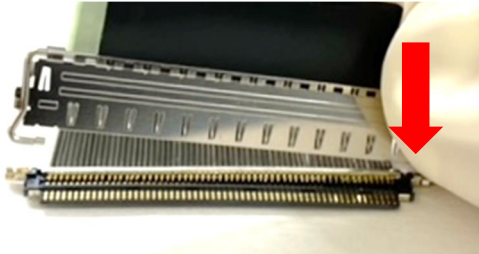
Photo.11 Assembly of Lock Bar Assembly
