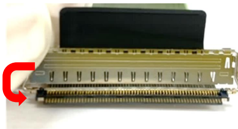
Photo.12 Assembly of Lock Bar Assembly
