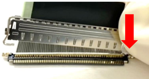
Photo.11 Assembly of Lock Bar Assembly
