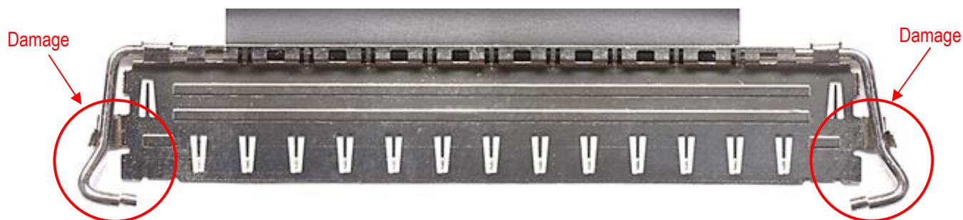
Photo.13 After Deformation Lock Bar Assembly
