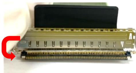
Photo.12 Assembly of Lock Bar Assembly
