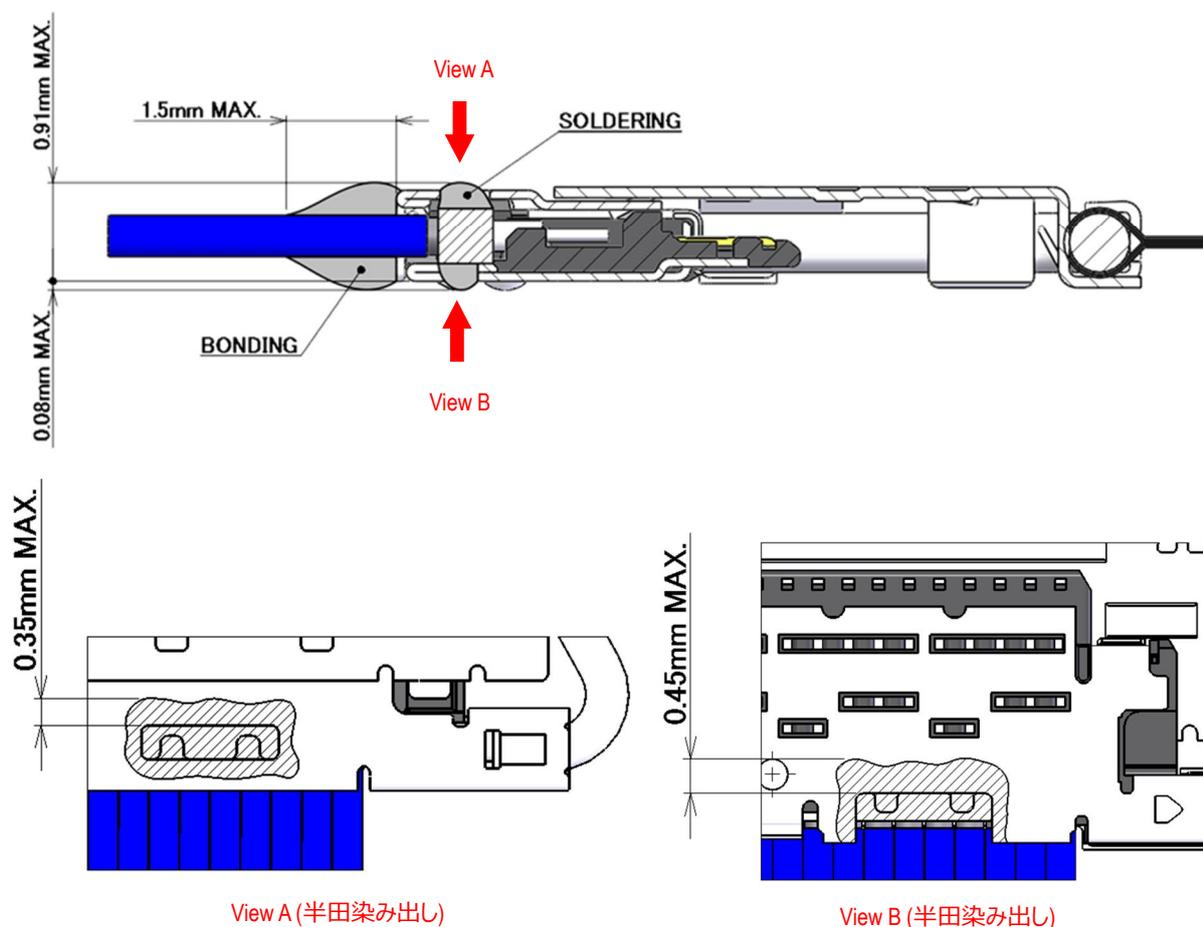
Fig.13 Soldering & Bonding
