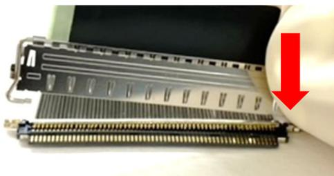
Photo.11 Assembly of Lock Bar Assembly
