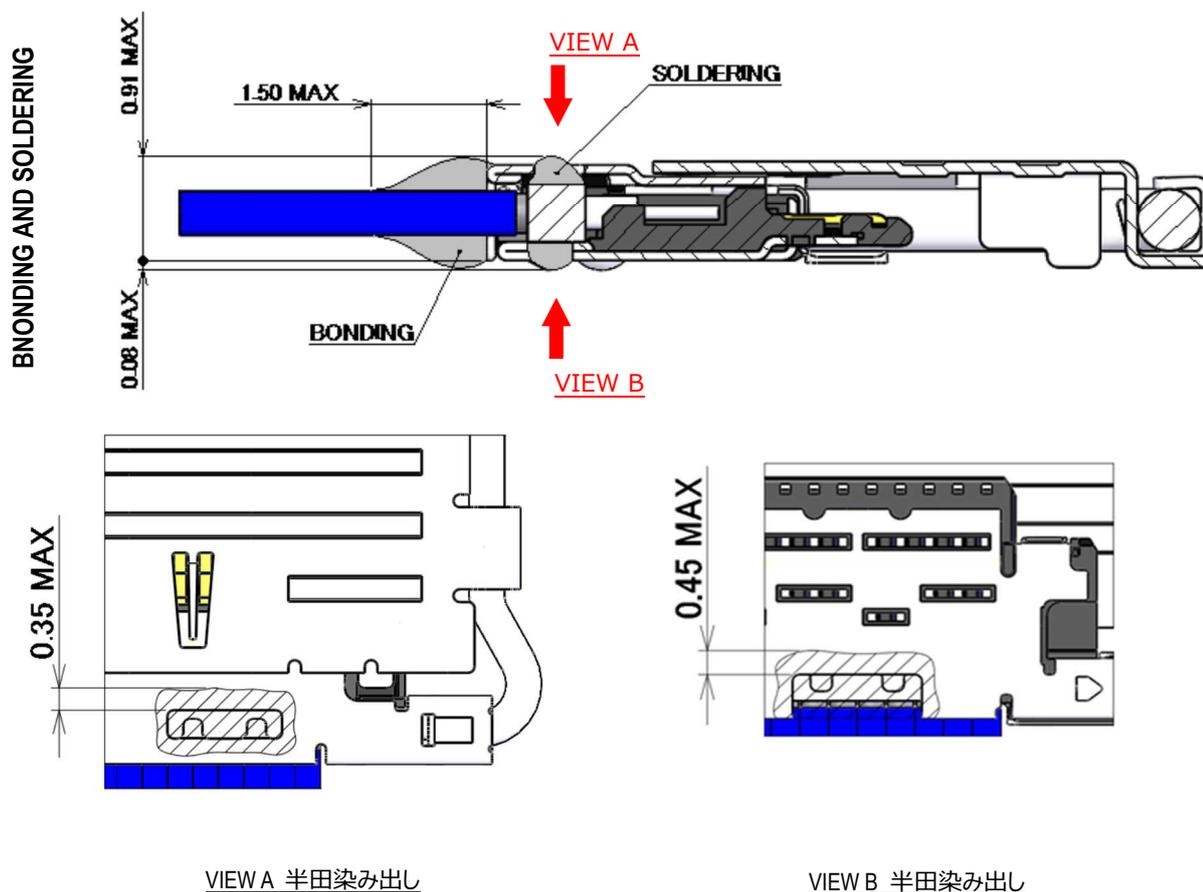
Fig.14 Soldering & Bonding
