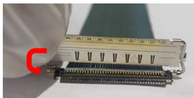
Photo.12 Assembly of LOCK BAR ASS'Y
