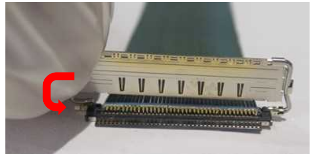
Photo.12 Assembly of LOCK BAR ASS'Y
