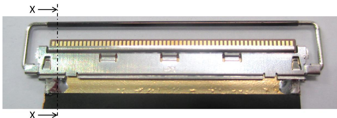
Photo. 3 Soldering of Shell and FPC
