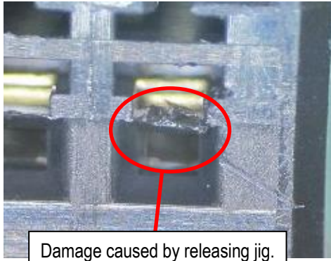
Fig42 Damage caused by releasing jig
