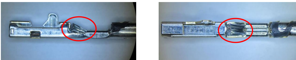
Fig 19 Excessive conductors out
