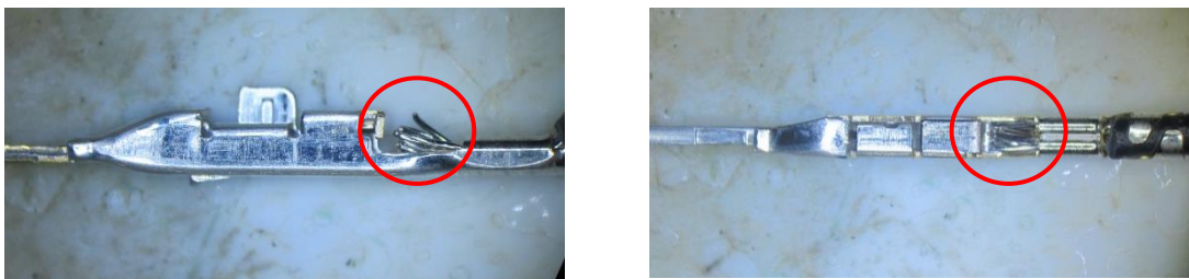
Fig 19 Excessive conductors out
