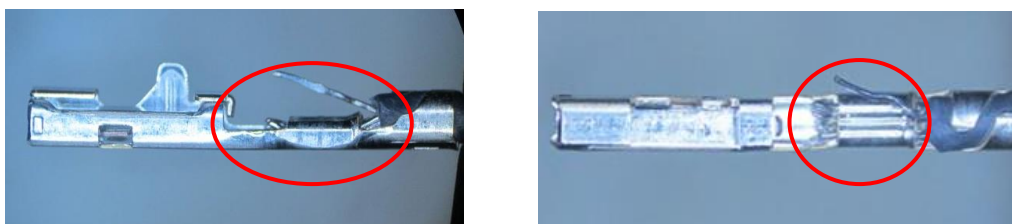
Fig 20. Incomplete conductors crimping
