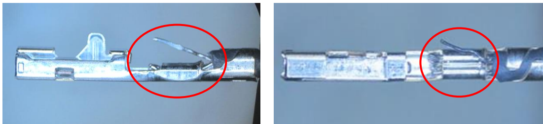
Fig.22 Incomplete conductors crimping
