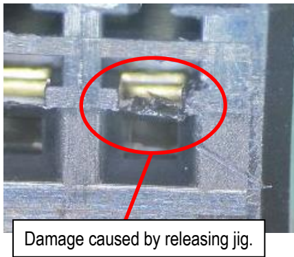
Fig.41 Damage caused by releasing jig
