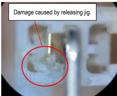
Fig31. Damage caused by releasing jig
