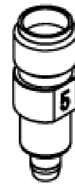
MHF 5 RECEPTACLE HIGH CYCLE ATTACHMENT PART NO. 90690-0001
