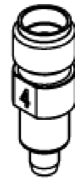
MHF 4 RECEPTACLE HIGH CYCLE ATTACHMENT PART NO. 90683-0001
