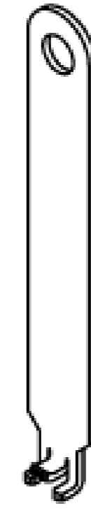
FRONT SIDE BACK SIDE MHF 4L (1.37) PUSHING AND PULLING TOOL PART NO. 90873-0001
